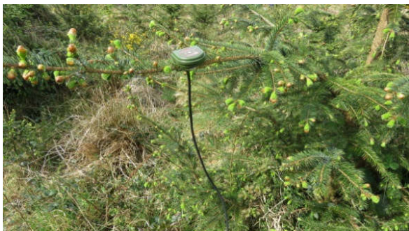
Photo 20 – microphone in position at Site Q
