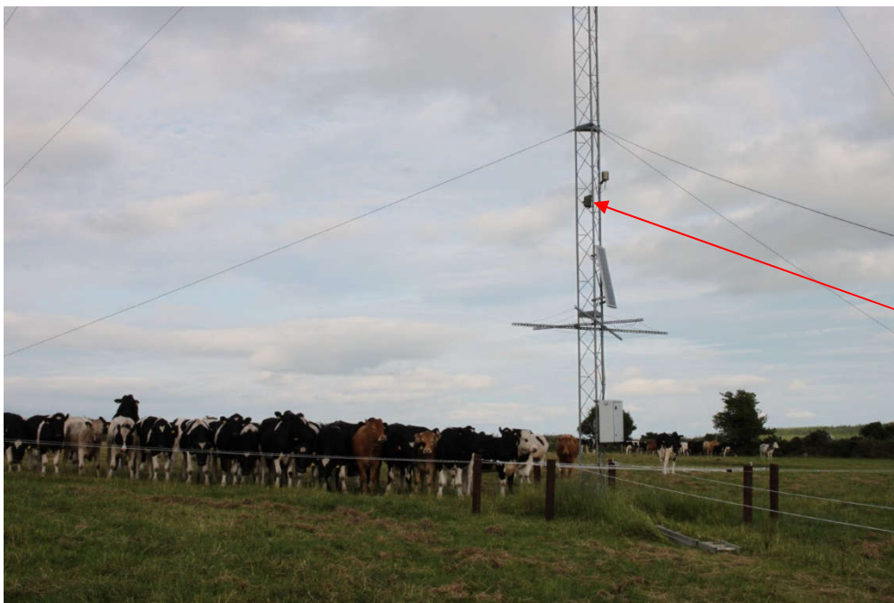
Photo 43 - Songmeter SM4 in position on anemometer
